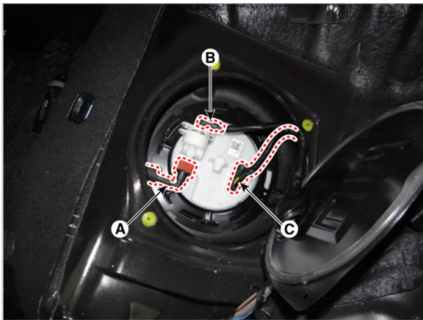
8. Remove the locking ring (A) by using the special service tool (B) [No.: 09310-B8100].
