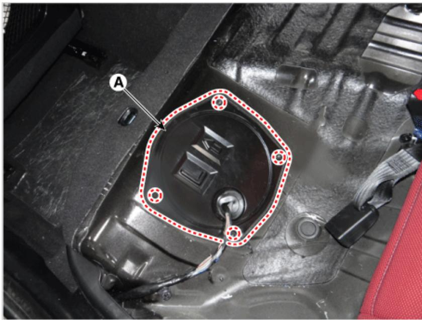
5. Disconnect the fuel feed quick-connector (A).
